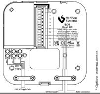
**Note:** Disconnect any Opentherm thermostat from the boiler and reconnect to "OT Thermostat" connections on the BCM.
